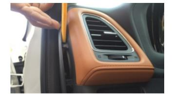
21. Carefully pry to disengage the clips and remove the driver's side button mounting panel.
