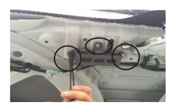
17. Attach the ground wire as shown.
