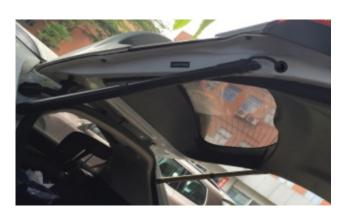
13. Using a wire puller or fish tape, carefully pull the wire harness through the wiring boot.
