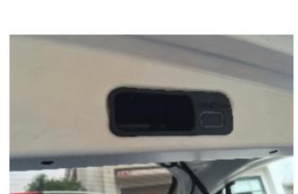
16. Remove the 3 bolts as shown. Install the control module/mounting bracket as pictured.
