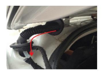
14. Using the wire puller or fish tape, pull the wire harness through the lift gate body structure as pictured.
