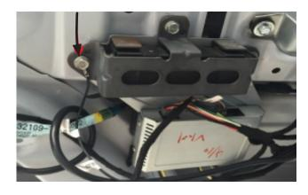
18. Route the main wiring harness forward, along the path indicated in the image.
