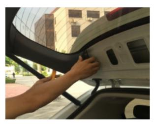
3. Carefully pry with a nylon trim tool to disengage the clips, and remove the lift gate interior door trim panel.
