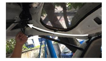
15. Remove the OEM pull handle cup from the lift gate. Install the supplied pull handle cup with open/close button into the location. Connect the wire harness and route the wire harness to the control module mounting location.
