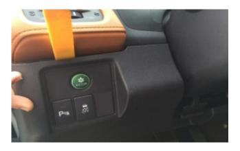
22. Remove the blank knock-out and mount the supplied open/close button in the location as pictured.
