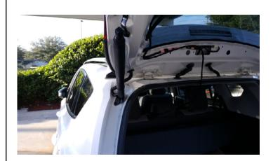
13. Remove the rubber plug from the lift gate above the lift motor. Carefully cut out the hole plug from the rubber cover.
