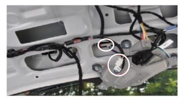
17. Install the main control module onto the door frame with the 2 supplied bolts, as pictured. Verify the bracket is tight and does not cause any rattles or other undesirable effects in the lift gate.
