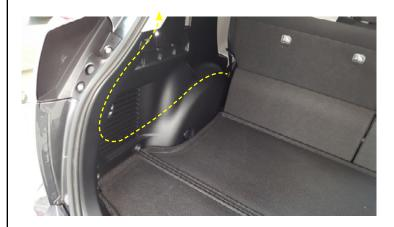
25. Carefully pull the main wiring harness through the harness boot and into the lift gate door.
