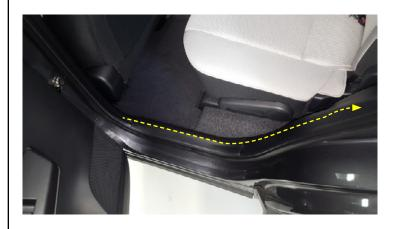
24. Using a fish tape or wire puller, pull the harness through the rear interior trim panel rearwards, and up towards the headliner.
