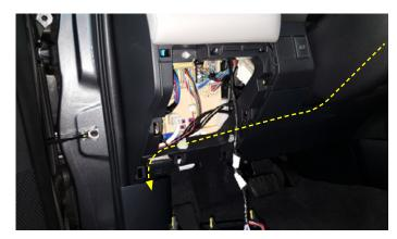
21. Mount the supplied Power Lift Gate Opener Switch into the factory knock-out location.
