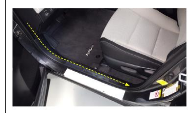
23. Continue routing the main wiring harness along the factory wiring harness towards the rear of the vehicle, underneath the scuff plate.
