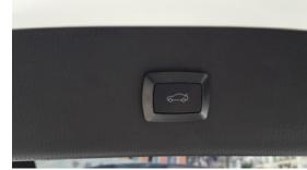
19. Mount the interior open/close button in the driver's side lower dash panel and secure with the nut. Connect to the wiring harness and reinstall the driver's side lower dash panel.
