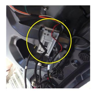
10. Locate the OEM outside opener switch connector, on the rear of the switch assembly. Disconnect the OEM connector, and connect our T-Harness in line with the outside opener switch.
