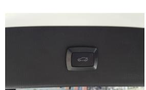
20. IMPORTANT: Prior to closing, ensure door panel is re-installed. Manually close the lift gate to initialize the Power Lift Gate System. Function test the system to verify proper operation.
