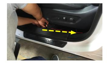
23. Continue routing the main wiring harness under the trunk floor, behind the panels up towards the headliner. Use a fish tape to help in pulling the harness through the factory wiring boot.
