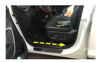
22. Continue routing the main wiring harness along the factory wiring harness towards the rear of the vehicle, underneath the scuff plate.
