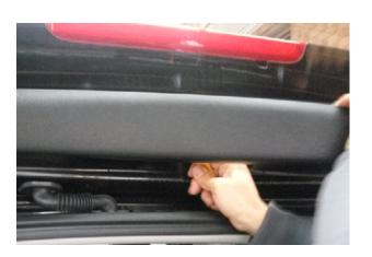
3. Carefully pull on the tailgate left and right side plaques to disengage the clips. Disconnect any connectors and remove the tailgate left and right side plaques.
