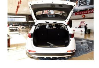
30. IMPORTANT: Prior to closing, ensure door panel is re-installed. Manually close the lift gate to initialize the Power Lift Gate System. Function test the system to verify proper operation.
