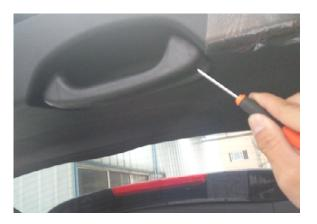
6. Remove cover and dismantle the handle. 7. Remove the plastic buckle from tailgate, near the locking mechanism. 8. Remove large tailgate plaque. 9. INstall the main control module onto the door frame with the clamp bracket, as pictured. Verify the bracket is tight and does not cause any rattles or other undesirable effectis in the liftgate. 10. Use the supplied t-harness for lock wire connection. 11. Use supplied t-harness for original button con-
