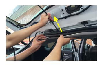
24. If necessary, use a wire pulling tool to route to tailgate.
