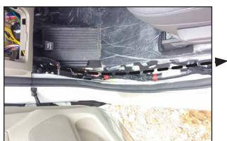
22. Locate the OBDII connector. Disconnect the connector from it's mounting location and connect into the supplied T-Harness. Mount the T-Harness connector into the factory location.
