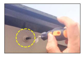
8. Disengage the claws and remove the cover for the lift gate mounting screw. Remove the screw.
