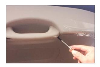
7. Using a screwdriver, carefully remove the plastic trim clip on the lift gate, near the latch.
