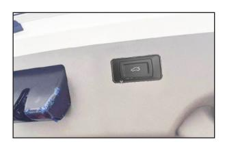
31. Reinstall the interior lift gate interior trim panel.
