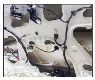
26. Connect wire clamp for unlock signal to OEM back button connector - RED WIRE.
