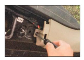
3. Carefully pull on the tailgate left and right side plaques to disengage the clips. Disconnect any connectors and remove the tailgate left and right side garnish.
