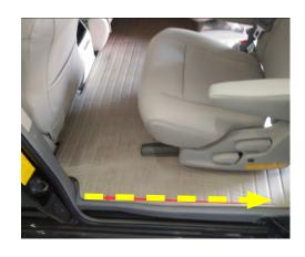
24. Using a fish tape or wire puller, pull the harness through the rear interior trim panel rearwards, and up towards the headliner.
