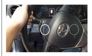
20. Connect the Canbus harness to the connector at the ignition key switch using the supplied T-harness. Route the wiring harness towards the driver's side under dash. Connect to the Power Transfer connector using the supplied T-harness, located at the fuse box. Then route the main wiring harness downward towards the kick panel.
