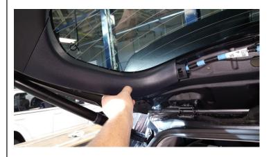
4. Insert a moulding remover into the slot and pry gently to disengage the clips on the back door trim panel. Pulling straight downward, disengage the rest of the clips and remove the back door trim panel.
