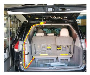
25. Carefully pull the main wiring harness through the harness boot and into the lift gate door.
