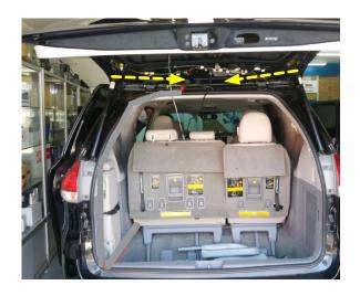
13. Remove the rubber plug from the lift gate above the lift motor. Carefully cut out the hole plug from the rubber cover.
