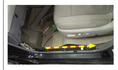
23. Continue routing the main wiring harness along the factory wiring harness towards the rear of the vehicle, underneath the scuff plate.
