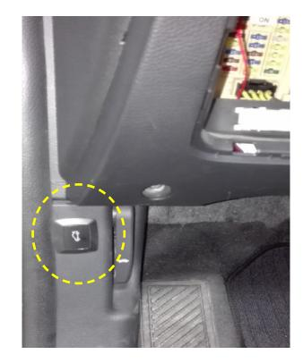
24. IMPORTANT: Prior to closing, ensure door panel is re-installed. Manually close the lift gate to initialize the Power Lift Gate System. Function test the system to verify proper operation.
