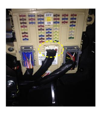
19. Route the main wiring harness along the factory wiring harness towards the rear of the vehicle, underneath the scuff plate.
